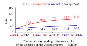
Fig. 13. Comparison of the values of the wear numbers for the right wheel in the symmetrical and asymmetrical wheelset guide stiffness configuration number 1
