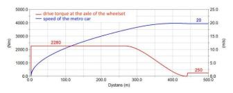
Fig. 9. Model metro wagon speed and driving torque at the axle of the wheelset as a function of distance [14]
