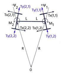
Fig. 8. Signs of angles of attack and tangential forces acting on bogie wheels on curved track
