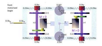
Fig. 5 Phenomenological model of the motor bogie [14]
