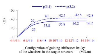
Fig. 15. Values of the quality factor for the solution with asymmetry of the stiffness of the wheelset guide for the wheelset number 3
