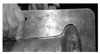
Fig. 4. Visualisation of wear on the wheel running surface [8]
