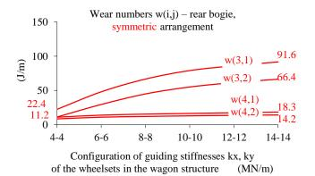
Fig. 11. Rear bogie wheel wear numbers with symmetrical wheelset guide stiffness configuration
