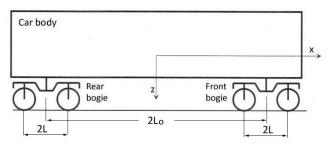
Fig. 3. Diagram of the structure of a metro car model
